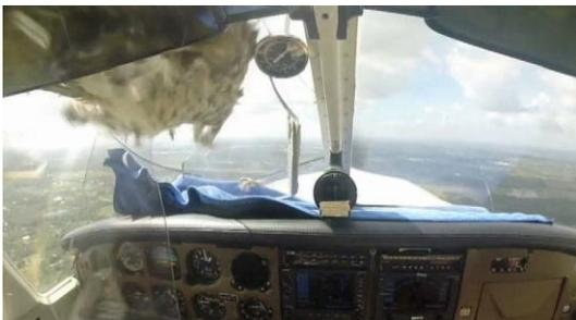
If involved in a bird strike, many pilots seem to forget the first and most important rule of flying: Fly the aircraft. If the weather is cool, consider warming the windshield to reduce the chances of it shattering if a bird were to hit. Also consider keeping shatterproof glasses/goggles on hand to wear when taking off or landing in areas with birds. If we en-
